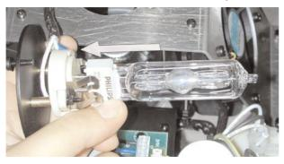
7) Replace the lamp assembly into its original position and replace and retighten the screws
