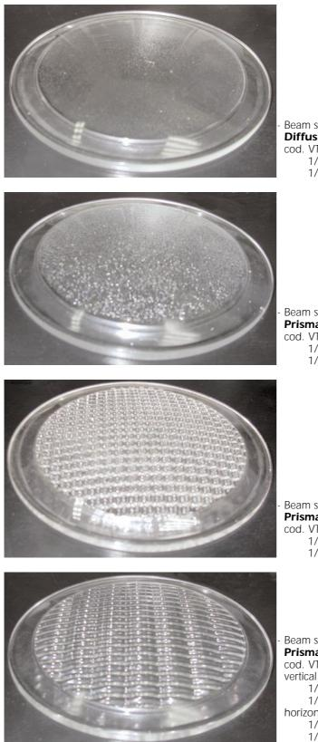
Beam shape: circular **Diffusion lense** cod. VT 171/3 1/2 peak angle: 9,5° 1/10 peak angle: 20°
