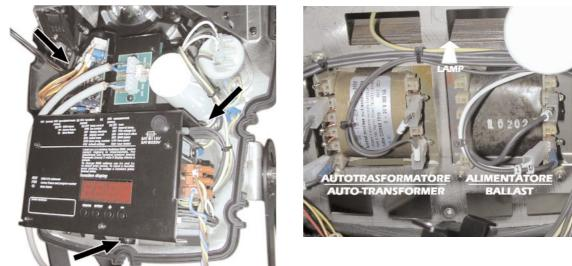
2) Select a voltage from amongst 100, 115, 208, 230 and 240V by removing cable n° 3 and moving it to the required voltage. To determine which is the correct tap, refer to the sticker located on the autotransformer.
