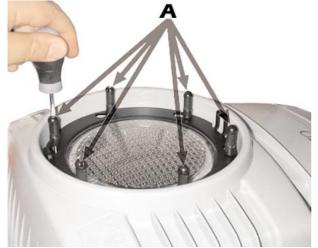
2) Rotate and remove the fixing ring.
