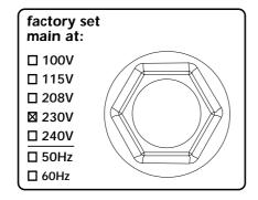
If the specified voltage and frequency do not match those of the country in which you are operating, follow the instructions in section 18 of this manual. "Altering the operating voltage and frequency" Incorrect voltage and frequency selection will detrimentally affect the operation of the projector.
