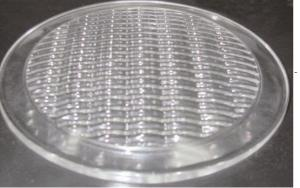
Beam shape: rectangular Prismatic outline/shaped lense cod. VT 171 vertical projection 1/2 peak angle: 24° 1/10 peak angle: 40° horizontal projection 1/2 peak angle: 55° 1/10 peak angle: 68°
